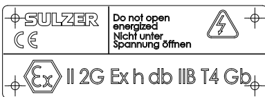
Figure 9b Nameplate ATEX
