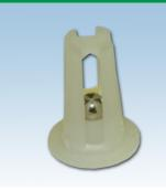
Check valves (non-return-valves) consist of a PP housing containing an 8 mm SS-ball. The stainless-steel ball prevents backflow of sludge into headers in case of damage to the membrane of the disc. Check valves alter the headloss characteristic of JetFlex<sup>®</sup> disc diffusers, so do not install discs with and without check valve in the same tank or on the same grid. Check valves work best if discs are installed using our clamp adaptors 90N or our rubber saddles, see above.
