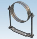
Pipe supports are made from stainless steel (ANSI 304/316) with adjustable height for laterals and headers in order to achieve optimum uniformity of aeration. Available sizes are for 4" and 6" laterals and headers as well as for DN100 and DN150 metric sizes. Please, call for details.
