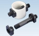
In order to join tube diffusers intended for square headers to 4-inch round headers there is a special connecting set available. Each set consists of 2 saddles and one connector threaded on both ends with 1" male threads.
