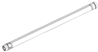
New diffuser body with grooves
